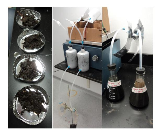
Figure 1: Samples taken from the mixtures for the first bench-scale reactors (left); bench-scale reactors, one with P&P AD sludge and one without, gas bags on the top and IV bags on the bottom for the purpose of manual leachate recirculation (center); blanks which have the same quantity of inocula as what was mixed into the reactors.
